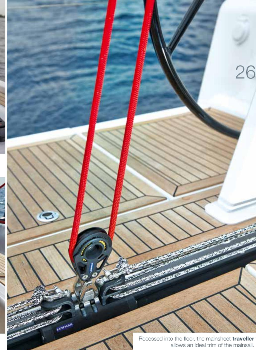
Recessed into the floor, the mainsheet traveller allows an ideal trim of the mainsail.
