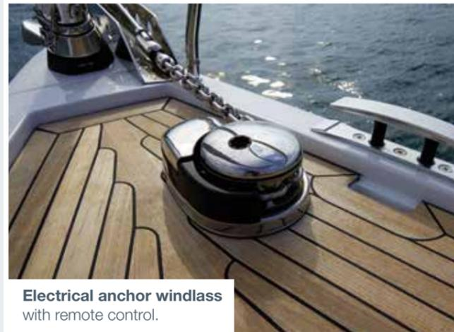
**Electrical anchor windlass** with remote control.
